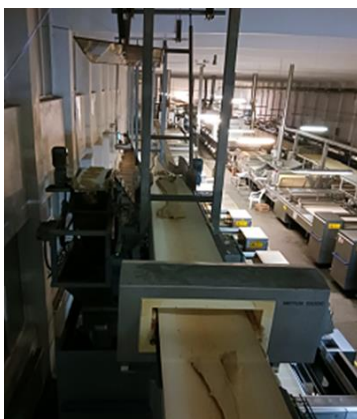
Fig. 12 Dough transport to hopper of rolling equipment
