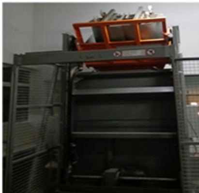
Fig.10 Dough lift up and overturning in kneading machine
