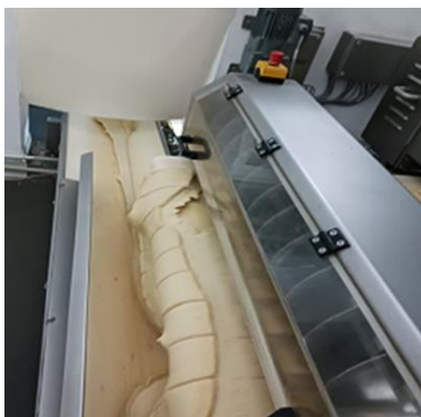
Fig. 11 Dough pieces exiting the kneading machine
