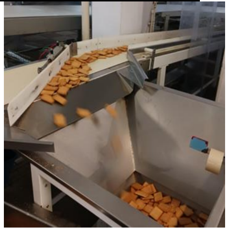
Fig. 25 Biscuits transport and vertical feeding up of packaging machine
