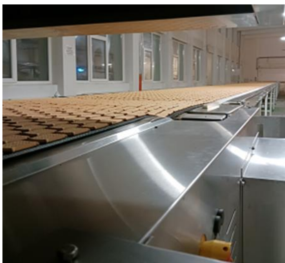
Fig. 21 Biscuits transport to the cooling area
