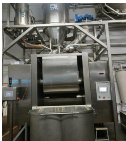
Fig. 9 Dough rest in mixer's mobile tubs
