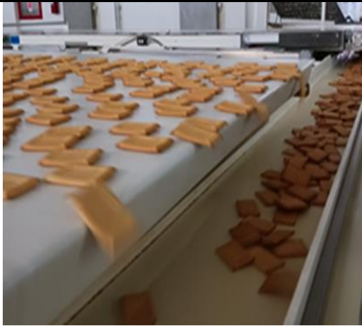
Fig. 25 Biscuits transport and vertical feeding up of packaging machine
