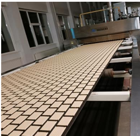
Fig. 19 Conveyor belt to oven
